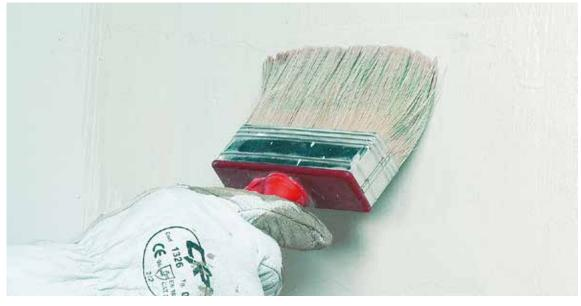
**TECHNICAL FEATURES:** BENFERPRIM is an acrylic polymer dispersion, designed to consolidate weak and dusty substrates. Once dry, it offers a good surface to Benfer tile adhesives, self levelling and waterproofing on all absorbent substrates common in building. It improves surface hardness and reduces water absorption to avoid a too fast water loss to the mortar applied on it.
