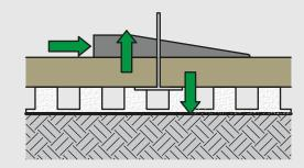
It follows the movements of the tile during the application for a perfect planarity of the floor.
