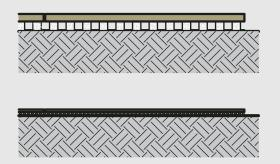
To be applied with a trowel in thickness from 3 to 20 mm.
