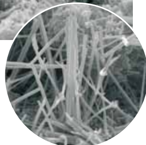
Magnified picture (10,000 X) of BETOCRETE C-16 nanocrystals
