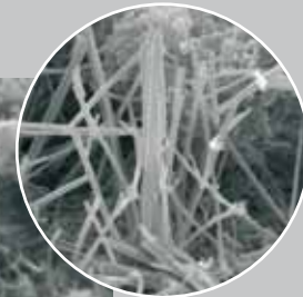
Magnified picture (10.000 X) of AQUAFIN®-IC nanocrystals.
